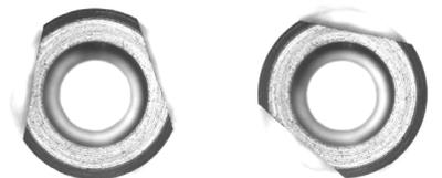
(c) Images using coaxial and back lights, and transparent jig
