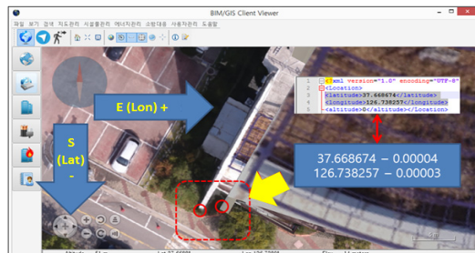
Fig. 13. Location correction between BIM model data and 3D model data using 5cm high resolution aerial image
