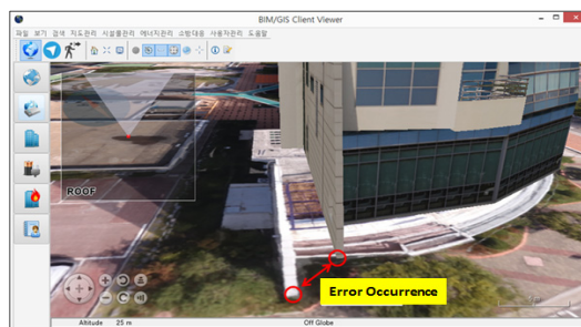
Fig. 12. Location error between BIM model data and 3D model data using 5cm high resolution aerial image
