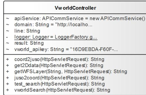
Fig. 10. Diagram for class controller to connect with BIM/GIS platform and V-world external data
