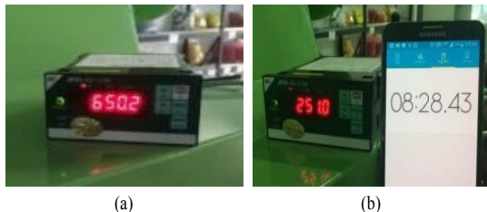
Fig. 18. Experiment to verify feed transfer capacity of AFTM no. 2 assembled automatic feeding system (a) Before feeding (b) After feeding
