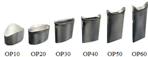
Fig. 1. Product sequence of square cup through multi-stages deep drawing process
