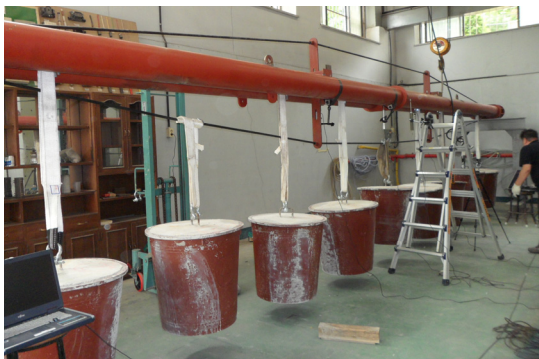
Fig. 7. Photo of cable wall system test
