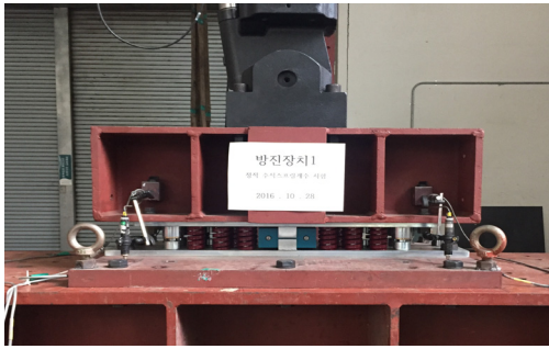
Fig. 5. Vertical static load test
