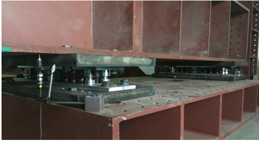
Fig. 8. Horizontal static load test (Longitudinal)
