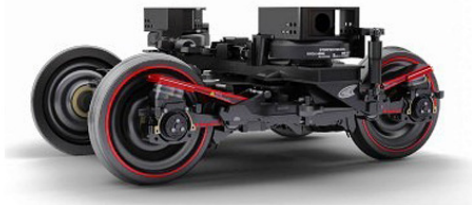
Fig. 1. Composite bogie developed by Kawasaki heavy industry [2].
