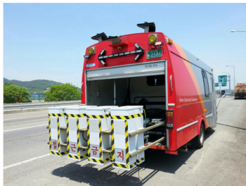
Fig. 2. GPR system used for bridge deck survey
