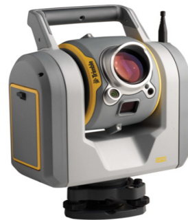
Fig. 3. Scanning Total Station
