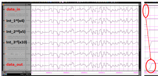
Fig. 8. Simulation results of the sampling rate up converter for UL0
