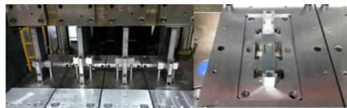
Fig. 4. Forging die for air vent manufacturing
