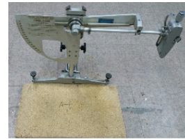
Fig. 3. Slip resistance test
