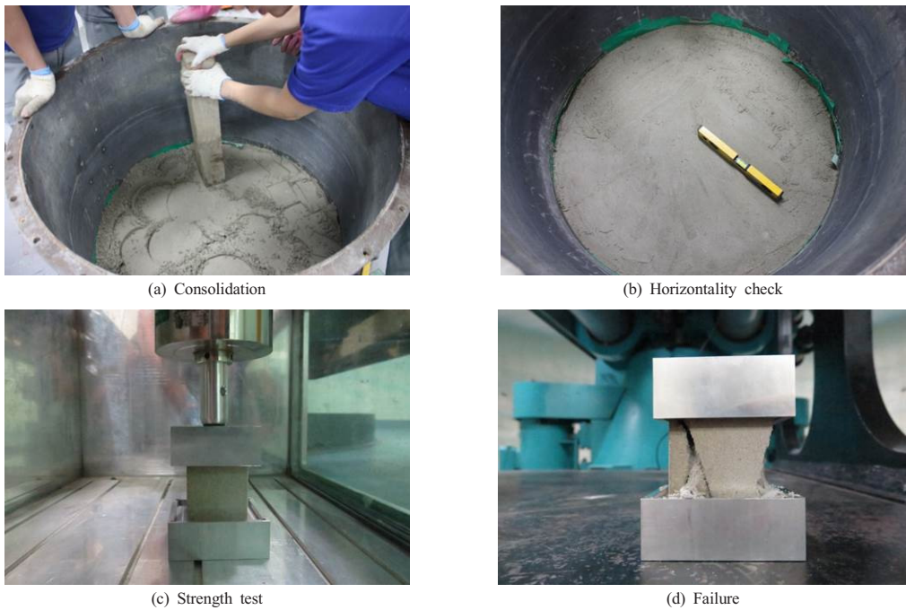
Fig. 6. Making and validating weathered rock for pile foundation
