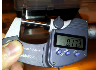
Fig. 5. The 173 \mu\text{m} -thick film whose thickness being measured by digital micrometer. (deposition time : 30 min)
