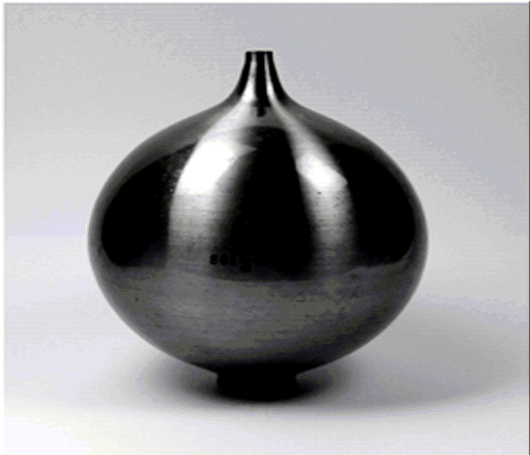
Fig. 1. The helmholtz type resonator
