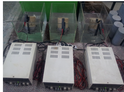
Fig. 2. Test method of NT build 492
