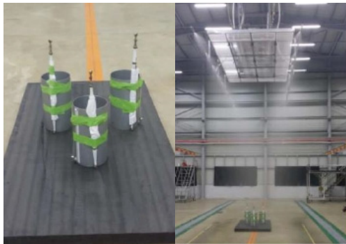
Fig. 10. Water Proof Test situation
