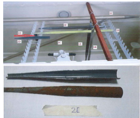
Fig. 11. Situation of Salt Fog Test
