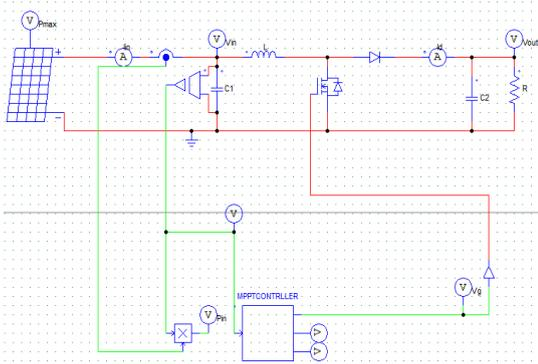
Fig. 14. PSIM circuit of Proposed MPPT method
