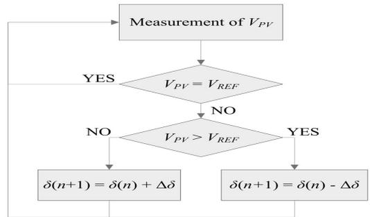
Fig. 4. Flowchart of the CV MPPT method
