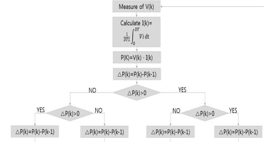
Fig. 13. Flowchart of Proposed MPPT algorithm
