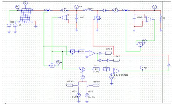
Fig. 8. PSIM circuit for P&O MPPT Control
