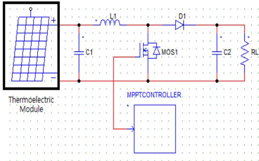
Fig. 10. Schematic diagram for Boost converter with TEM
