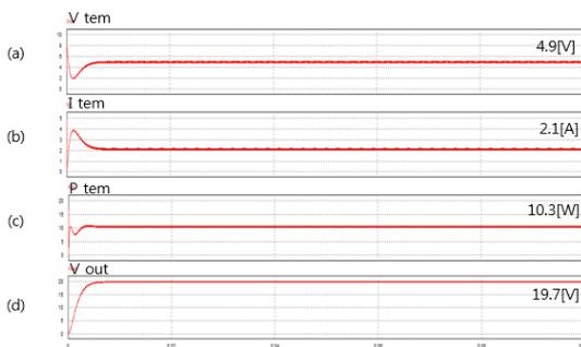
Fig. 7. Simulation Result constant voltage MPPT control
