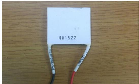
Fig. 17. TEM module used in the implementation
