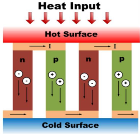
Fig. 1. Operating Principle of a Thermoelectric Module
