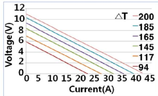
Fig. 2. V-I Characteristic of the thermoelectric module
