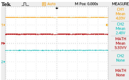
Fig. 18. Implementation result of proposed MPPT method
