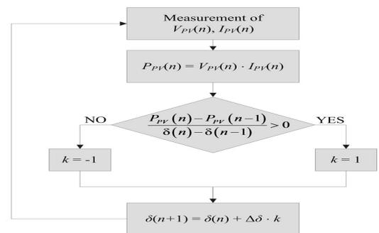
Fig. 5. Flowchart of P&O algorithm
