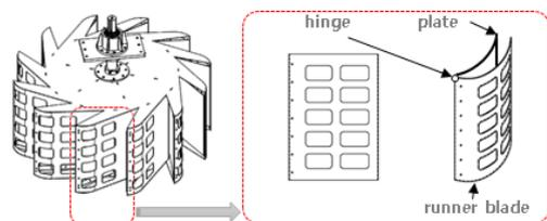
Fig. 3. Drag force type vertical axis hydro turbine
