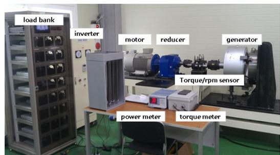
Fig. 6. Equipment configuration of generator efficiency test
