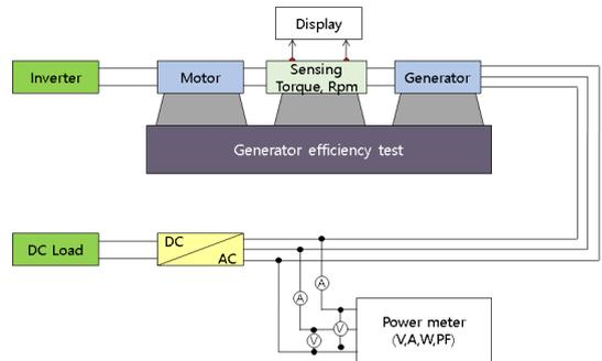
Fig. 5. Configuration diagram of generator efficiency test
