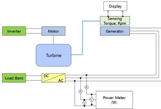
Fig. 7. Configuration diagram of electric energy test
