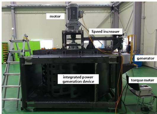
Fig. 8. Equipment configuration of electric energy test
