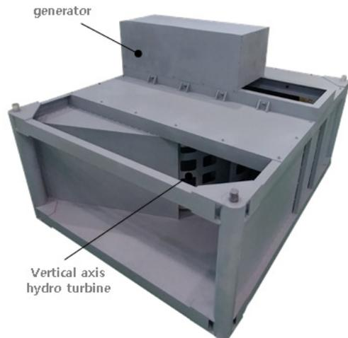
Fig. 2. Prototype of integrated power generation device
