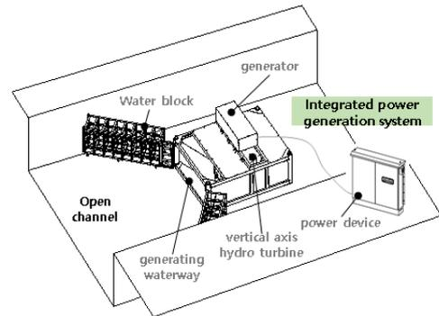
Fig. 1. Overview of integrated power generation system
