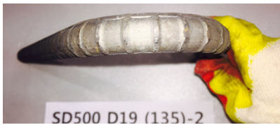
Fig. 3. Surface condition after bending test
