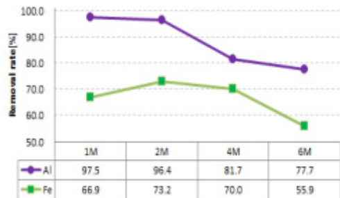
Fig. 2. Fe and Al removal rate after leaching with H 2 SO 4
