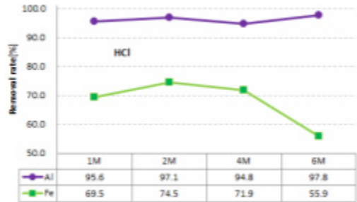
Fig. 5. Fe and Al removal rate after leaching with HCl
