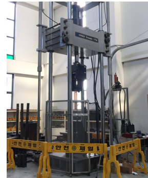
Fig. 1. 1,000 kN UTM at KICT
