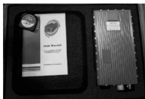
Fig. 5. DGPS & gyro sensor
