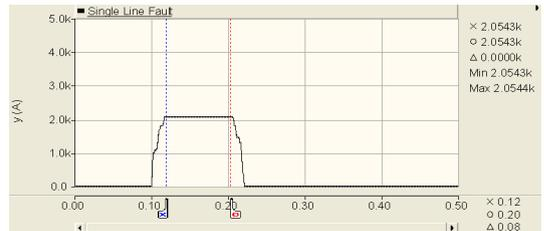
(a) Ground fault current[kA]
