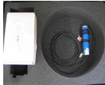
Fig. 5. Ultrasonic water-level meter
