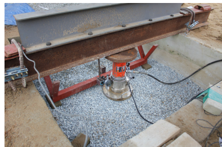
Fig. 9. Plate load bearing test
