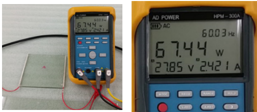
Fig. 9. Measurement of heating value of a non-patterned Low-e glass(100mm×100mm)
