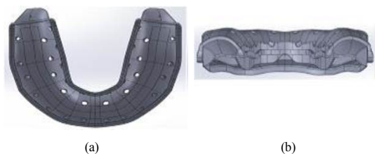
Fig. 2. Modeling of vacuum oral cleaner's inner part: (a) top view; (b) front view
