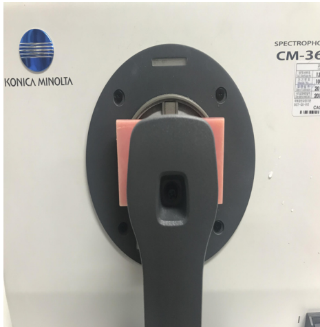
Fig. 4. Evaluating color of washed specimen
