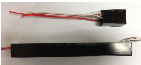
Fig. 7. Comparison of size of high-pressure equipment (Above: developed, below: conventional high pressure device)
