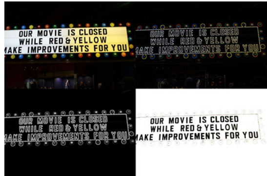
Fig. 3. Original image on up-left, edge detected image on up-right, gradient orientation image on bottom-left, and stroke width transformation image on bottom-right
