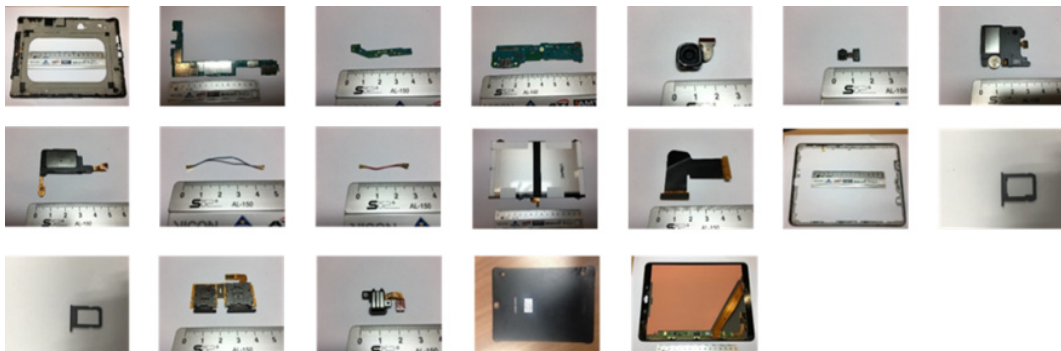
Fig. 1. Components of the tablet PC
