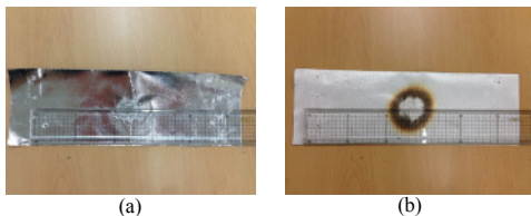
Fig. 3. Result of KS K 0583 (a)AL foil side (b)Glass fiber side
