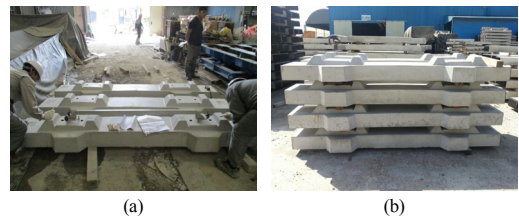
Fig. 5. Production of wide sleepers for quick-hardened concrete track (a) Inspection (b) Final products
