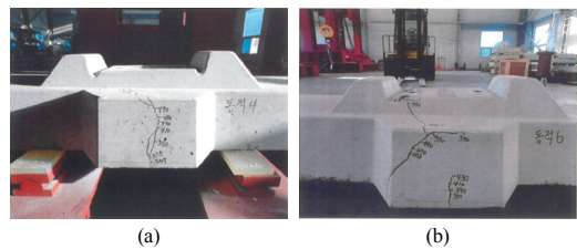
Fig. 13. Results of crack propagation after dynamic tests (a) S-RB: No.18 (flexural failure) (b) S-RB: No.19 (flexural-shear failure)
