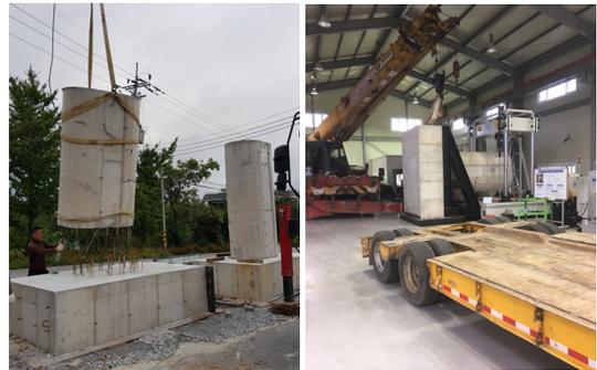
Fig. 19. Manufacture and setup of test specimen
