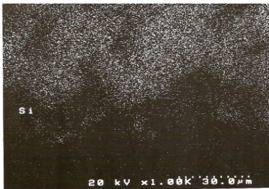
Fig. 9. EDX Si dot pattern of the porous SiC (upper) / Ag (lower) interface.
