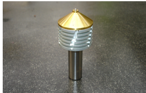
Fig. 1. Tool shape of FSW
