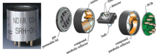
Fig. 5. Exploded View of Gas Cell
