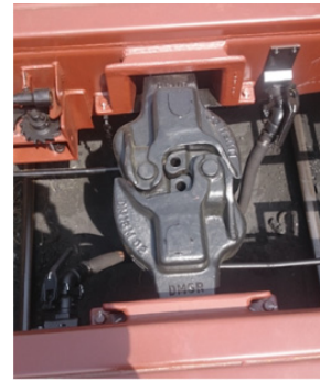
Fig. 1. Connection of freight coupler(AAR Type)
