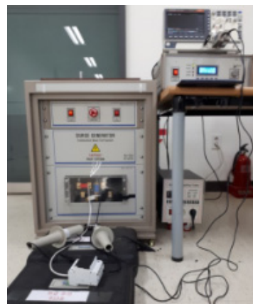
Fig. 7. Experiment setup for combination wave generator and measurement device
