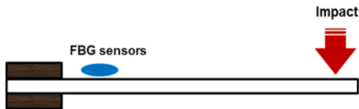
Fig. 3. Free vibration test of cantilever beam for measurement of acceleration
