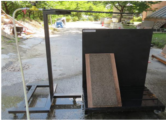
Fig. 4. Simulation test of rainfall intensity
