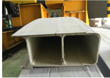
Fig. 12. Void section fracture mode
