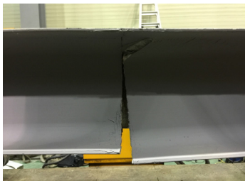
Fig. 16. Connected solid section fracture mode
