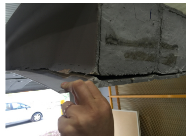
Fig. 18. Sand coating solid section fracture mode
