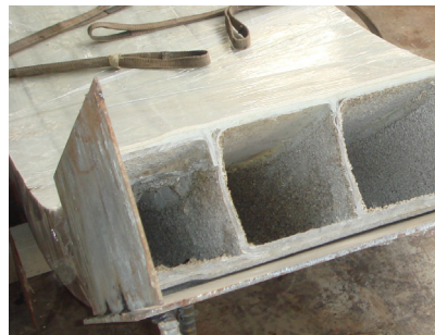
Fig. 5. Sand coating solid section
