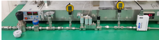
Fig. 9. Block Valve CV Test
