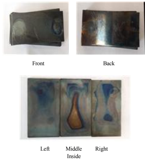
Fig. 9. Surface condition of specimen after annealing at 700 ℃.
