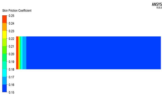
Fig. 15. Skin friction coefficient contour at pipe wall
