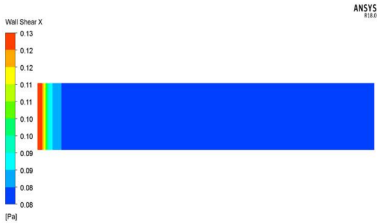
Fig. 14. Wall shear stress contour at pipe wall
