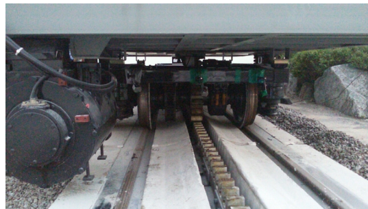
Fig. 22. Interface between bogie and track
