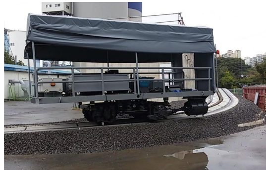
Fig. 21. Test vehicle of 1-bogie-and-1-carbody on the test track
