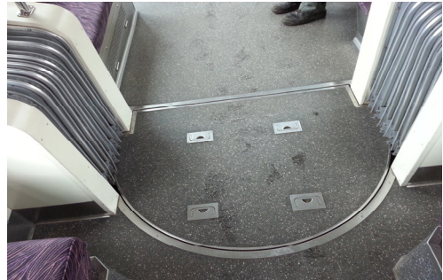
Fig. 16. Articulation in a tram
