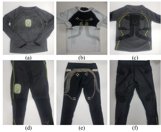
Fig. 25. Developed Self-trainer Fitness Wear Based on Silicone-SWCNT Sensor
