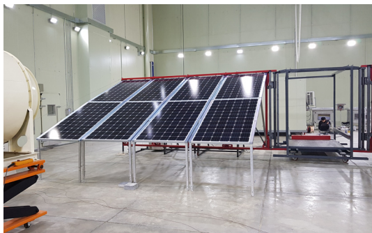
Fig. 14. Wind load Test(Front)
