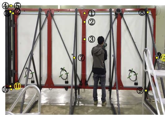
Fig. 13. Location of Strain gauge test
