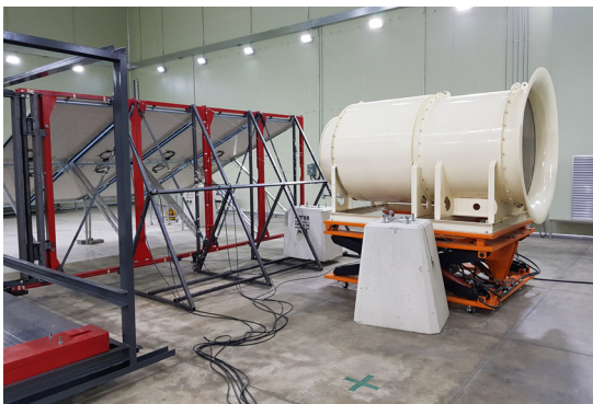
Fig. 15. Wind load Test(Back)
